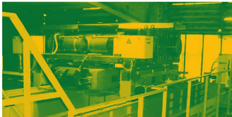
35 t Twin Drive Crane for Smelting Plant
